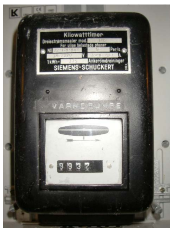
Fig. 1 Old electricity meter. The thin metal disc in the window rotates in the arrow's direction. Number of rotations indicates energy consumption. Modern meters blink and release electrical pulses which are monitored by computer.
