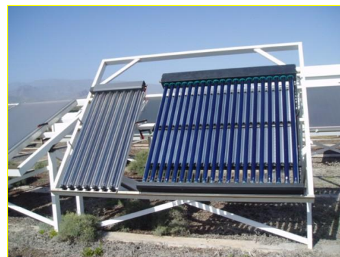
Figure 4. LABSOL: Solar collector test facility. The high direct radiation conditions makes ITC site at Pozo Izquierdo an excellent testing platform for high temperature solar thermal systems, and very suitable to host a solar furnace. One example is the Solar Collector Test Laboratory LABSOL, a platform TESTS for components of RES systems, first ENAC-qualified laboratory in Spain, and well positioned within the European context. LABSOL is providing services related with: (1) testing of solar cells; and (2) quality of photovoltaic plants.
